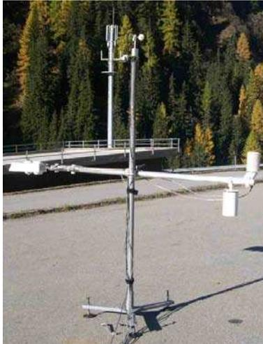
Fig. 1a. Mobile radiation balance station.
