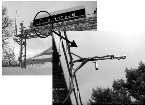
Fig. 4 Observational instruments set at Miyadai, a mountain pass of the national highway, 112.
