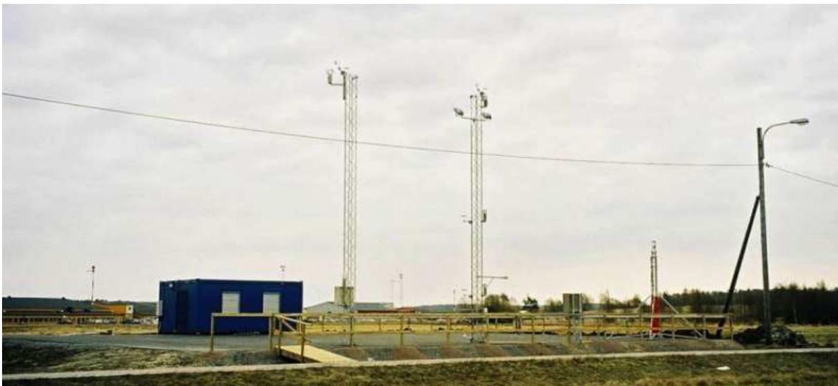
Fig. 1. The asphalt surface at Sävemåla as seen from the north-west. The sensors in the asphalt are near the right tower towards the centre of the surface. The two towers carry most of the instrumentation used in the study. The road is seen as a grey line in the foreground.
