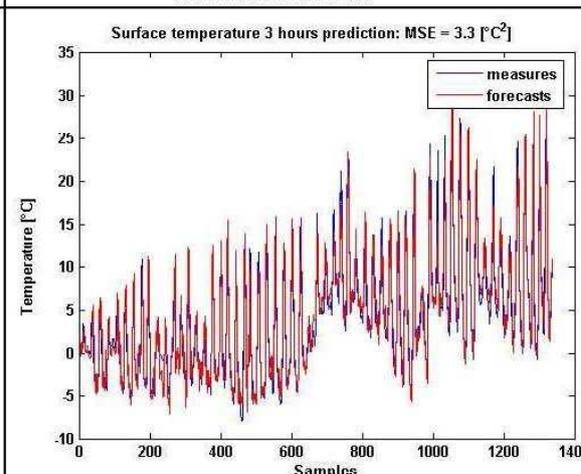
Fig. 8 d. RST prediction three hours ahead using selected predictors plus SMHI prognosis.
