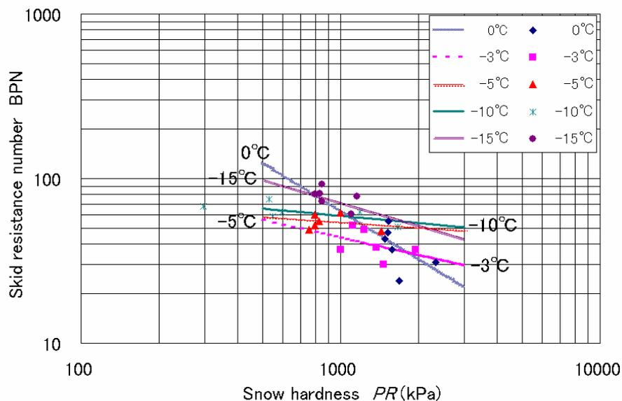
Fig. 4. Relation between the snow hardness and the skid resistance number.
