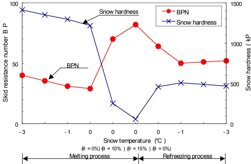
Fig. 6. Variation of the properties of snow in melting and refreezing process.
