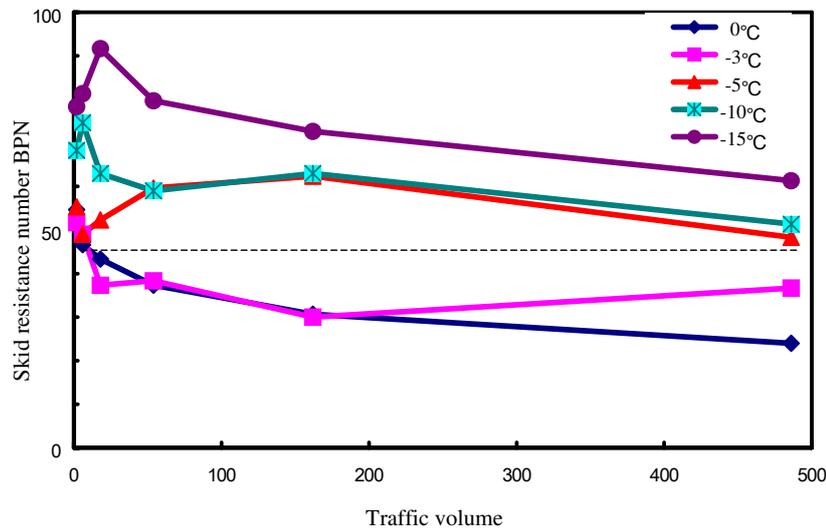
Fig. 3. Relation between the traffic volume and the skid resistance number.
