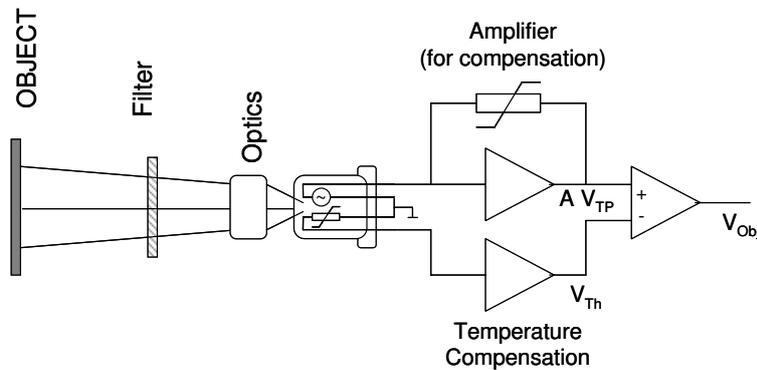
Fig. 2. Analogous Ambient Temperature Compensation
