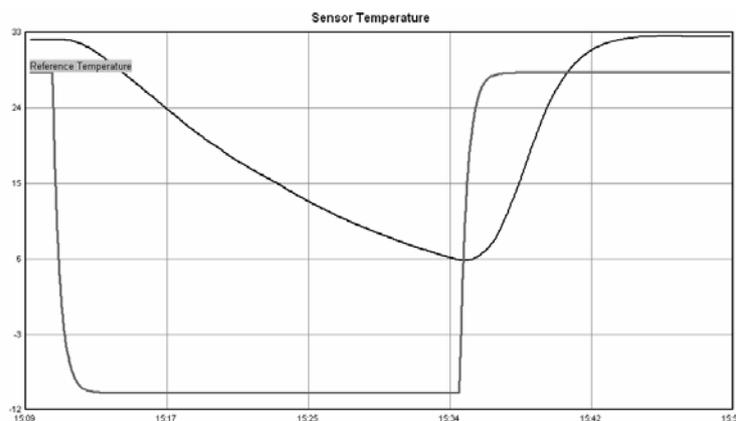
Fig. 5a. Sensor temperature change due to change of reference temperature.
