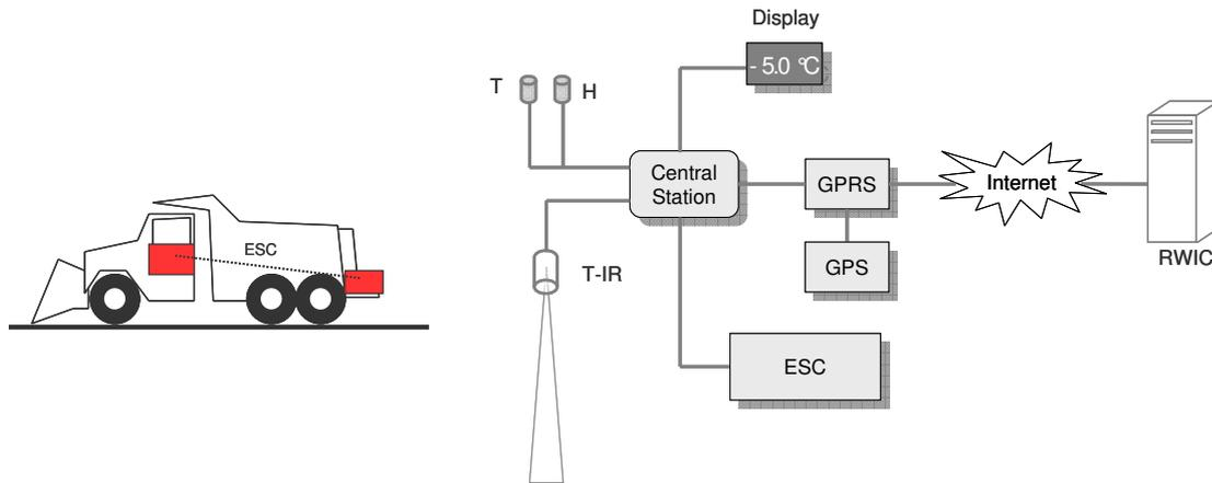
Fig. 1. Mobile Weather Station - System Overview
