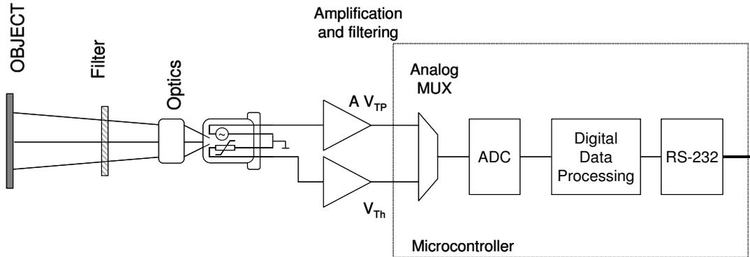
Fig. 3. Digital Ambient Temperature Compensation
