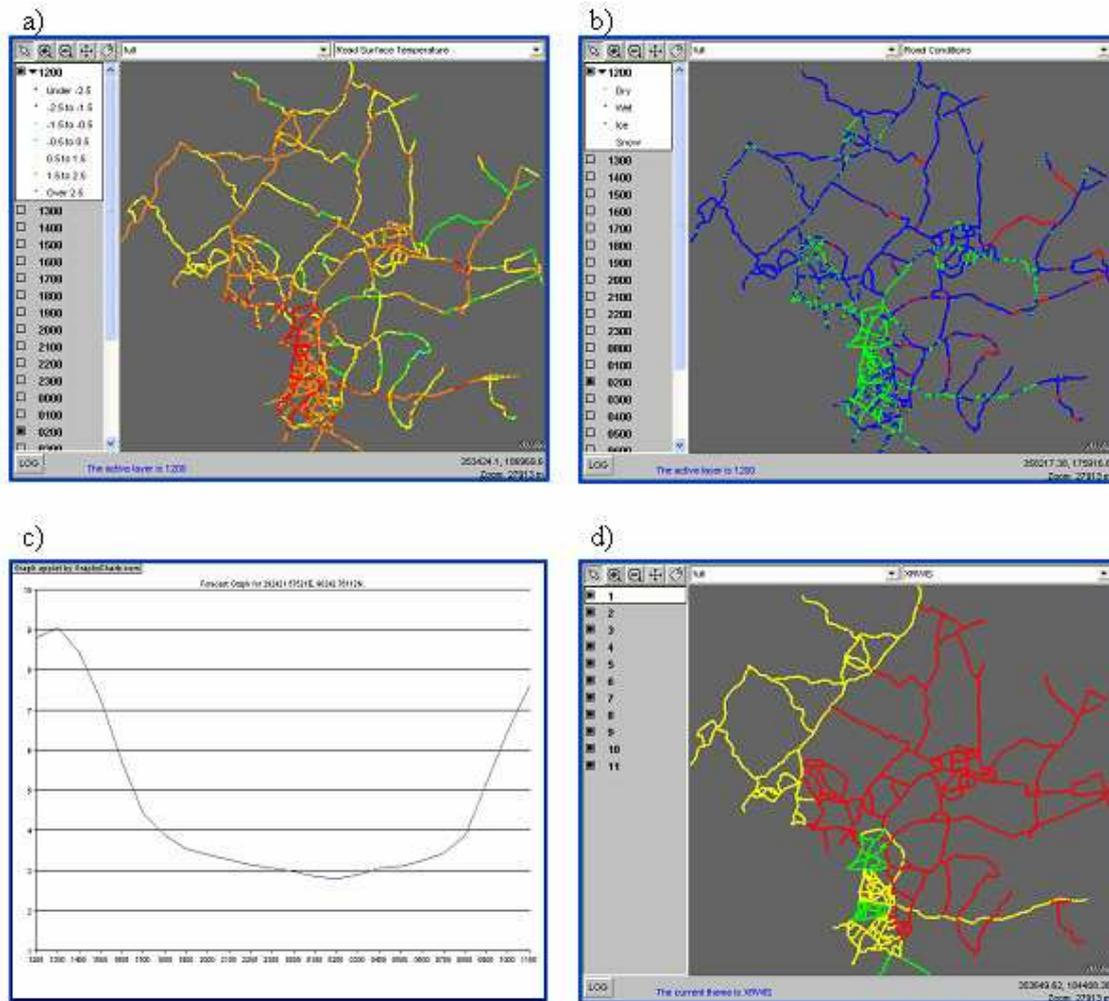
Fig. 1. Sample South Gloucestershire XRWIS output showing a) forecast road surface temperature, b) forecast road surface condition, c) forecast curve showing site specific variation in road surface temperature and d) traffic light colour-coded decisions; Red – route requires treating, Amber – standby (watch forecast) and Green – no action required.
