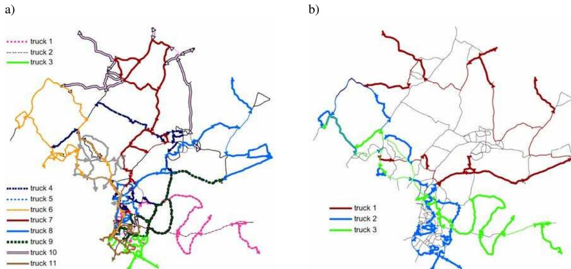
Fig. 4. Acquired solutions from the memetic algorithm for the CARP instances shown in Figure 3 for a) cold night and b) marginal night. A thick line denotes that truck should treat the road where as a thin line denotes the truck travels without service on the road.
