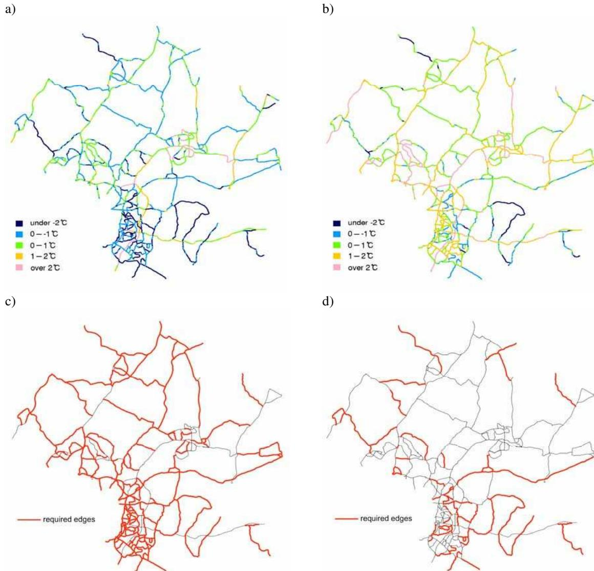
Fig. 3. Temperature distributions in South Gloucestershire, UK on a) a cold winter night and b) a marginal winter night. These temperature distributions are then translated into required edges in c) and d) respectively.
