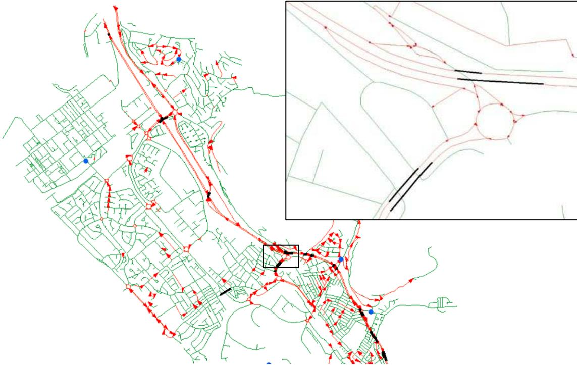
Fig. 2. Sample 'commercial, off the shelf' vector road network data suitable for use in salting route optimisation algorithms. Inset shows the finer detail of traffic restriction orders such as one-way streets (arrows), dual carriageways, intersections and bridge decks (bold).
