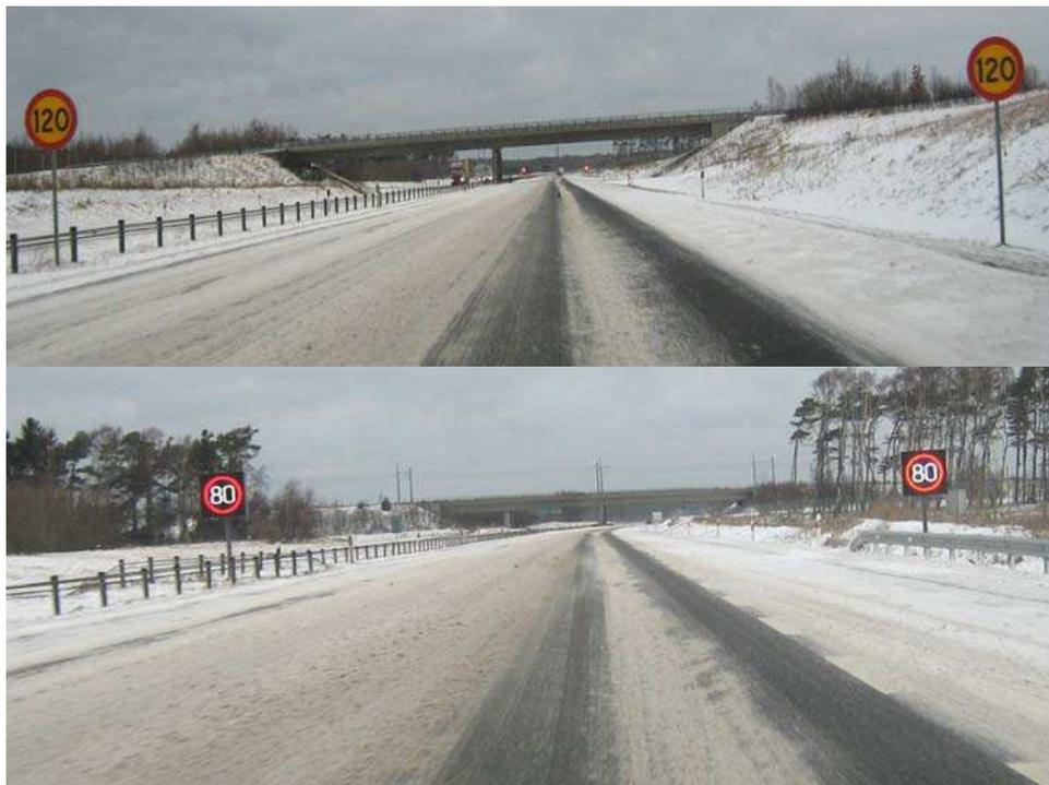
Fig. 2. Variable speed signs give up to date speed according to the prevailing road conditions along the road compared to the fixed speed sign.
