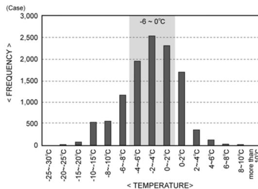
Fig. 5. Frequency of winter accident caused by slippery roads by temperature
