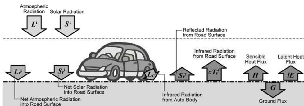
Fig. 6. Conceptual diagram of heat transfer at road surface
