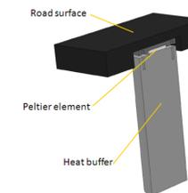
Figure 4: Cooling element used in Passive-BIRDS
