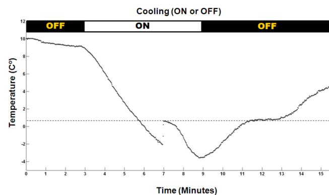
Figure 1: Temperature pattern during a freezing process produced with Active-BIRDS. Ice formation occurs at  $t = 7$  min and is detected due to the distinct temperature pattern.
