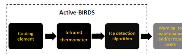
Figure 3: Schematic overview of the process chain involved in Active-BIRDS
