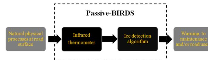
Figure 2: Schematic overview of the process chain involved in Passive-BIRDS
