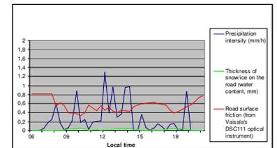
Fig. 7. Road weather observations at Vaskisalmi station (about 4 km west of Helsinki city center) on 8 February 2007 06-20 local time: precipitation intensity, thickness of snow/ice on the road as well as road surface friction measured by Vaisala's DSC111 optical instrument (data source: the Finnish Road Administration).
