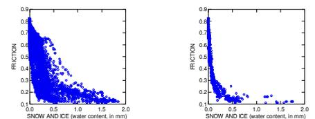
Fig. 8. Scatter plot of friction vs. the sum of snow and ice (water content in mm) on the road. Based on DSC111 observations in Utti (in southeastern Finland) during winter 2007/08. The left figure includes all observations, the right figure covers those cases when road surface temperature was below -5°C (data source: the Finnish Road Administration).
