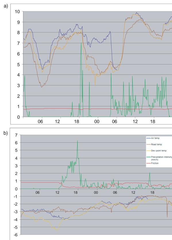
Road weather observations at Palojärvi (30 km northwest from Helsinki) on a) 10-11 November and b) 23-24 November 2008. The measurements include road surface friction measurements by Vaisala's DSC111 optical instrument (Finnish Road Administration).
