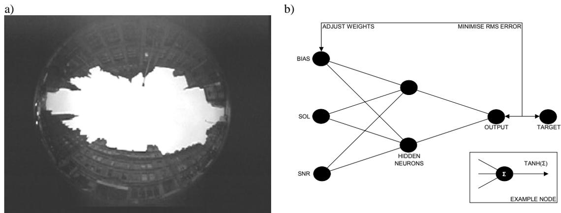
**Figure 2** a) Sample fisheye imagery and b) Artificial Neural Network used to calculate the sky-view factor by GPS proxy. SOL is the number of visible satellites used in the position solution whereas SNR is the sum of signal to noise ratios of available satellites.
