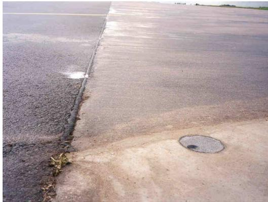
Figure 6: Water film sensor and the surrounding paved area. The sensor has dried-up even though the paved area is still moist.
