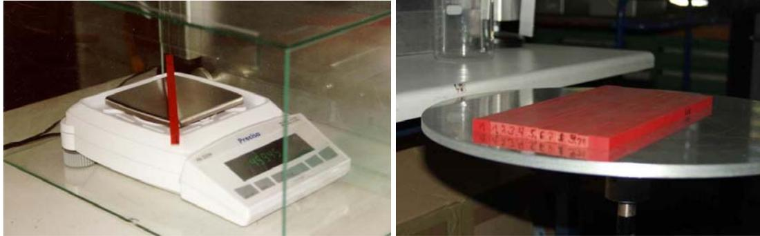
Figures 12 and 13: Plastic strips on the scales and under the jig for determining the water film thickness and the uniformity of application
