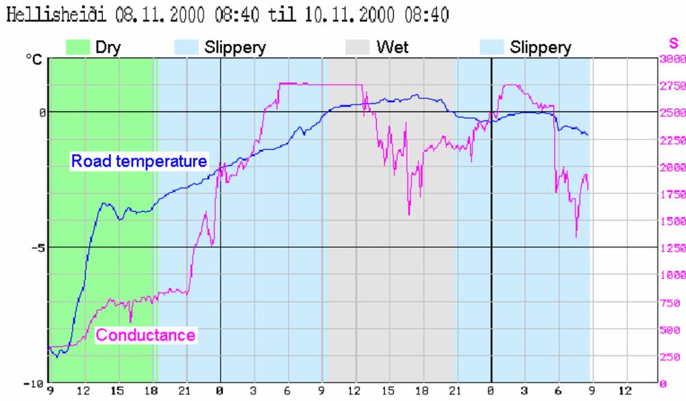
Experiments in measuring road surface conditions were not done for some time, but now a revised version of the method is ready, and five measuring devices will be put in place near Reykjavik in November 2003. The main changes in the new version are a new, electronically controlled reader for the measuring devices in the road surface and a revised technique for placement of the devices in the surface of the road. Plans call for presenting the findings of the new test in the spring of 2004.
