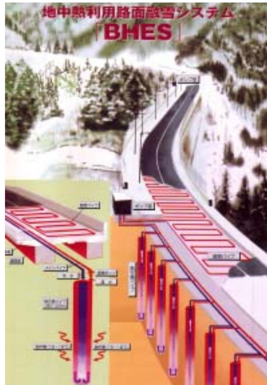
Fig.3 Borehole heat exchange system 3)
