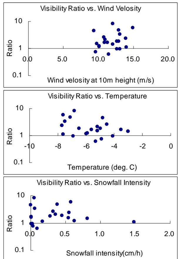
Figure 7 Visibility ratio (visibility at a height of 2.4 m : visibility at a height of 1.2 m) vs. weather factors. Top: wind velocity. Middle: air temperature. Bottom: snowfall intensity.
