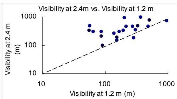
Figure 6 Comparison of visibility at 2.4 m and 1.2 m above the road. The dotted line indicates a visibility ratio of 1, i.e., where visibility at 2.4 m and 1.2 m are equal.
